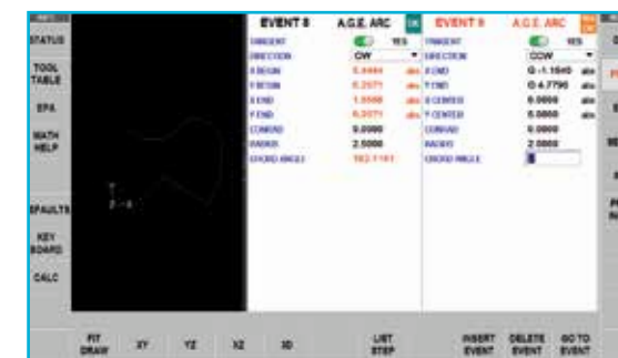
Auto Geometry Engine® software to fill missing data for you as you program
